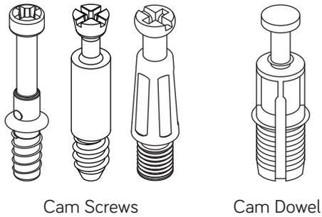
Turn the CAM SCREW or gently tap the CAM DOWEL until the shoulder is against the surface of the part.
