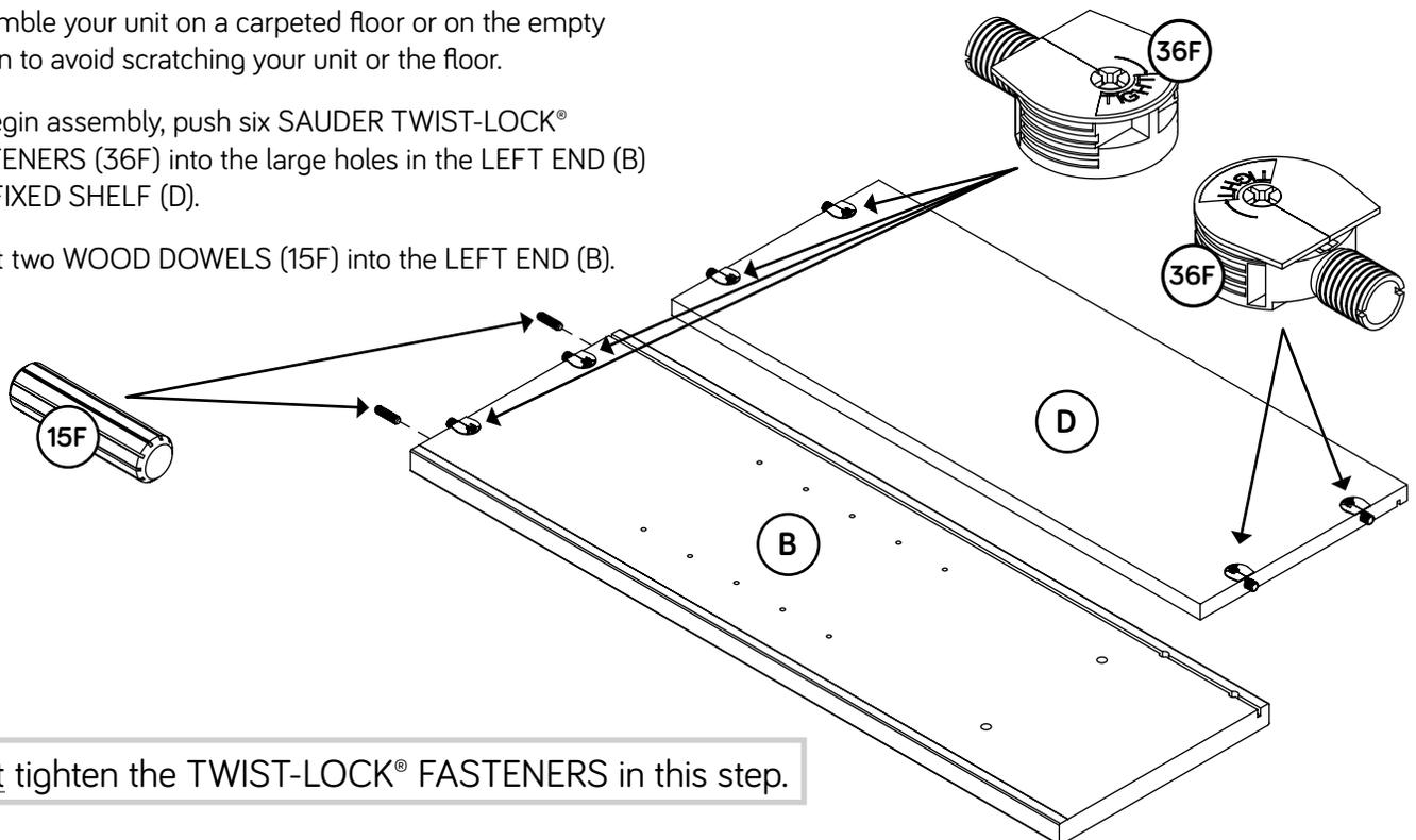
Do not tighten the TWIST-LOCK® FASTENERS in this step.
