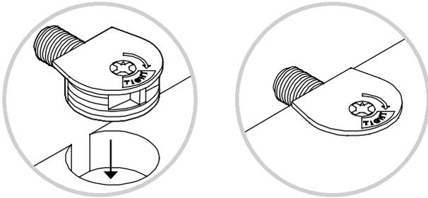
2. 1. Insert the dowel end of the FASTENER into the hole of the adjoining part.
