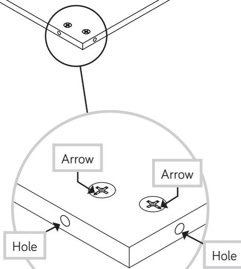
The arrow in the HIDDEN CAM must point toward the hole in the edge of the board.
