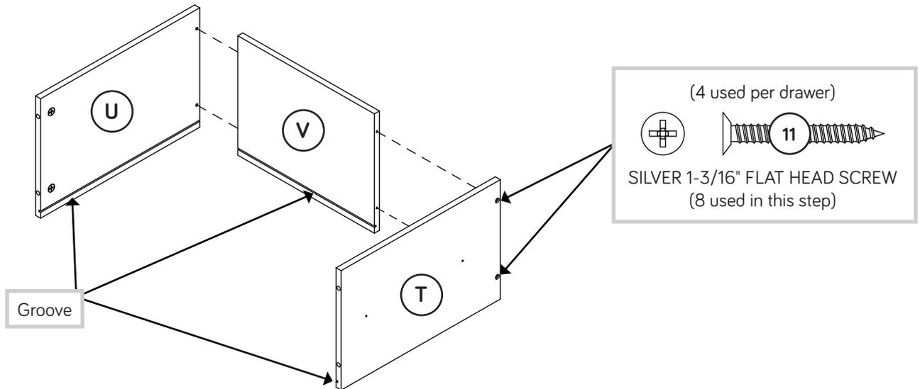
Fasten the LARGE DRAWER SIDES (T and U) to the LARGE DRAWER BACK (V). Use four SILVER 1-3/16" FLAT HEAD SCREWS (11).
