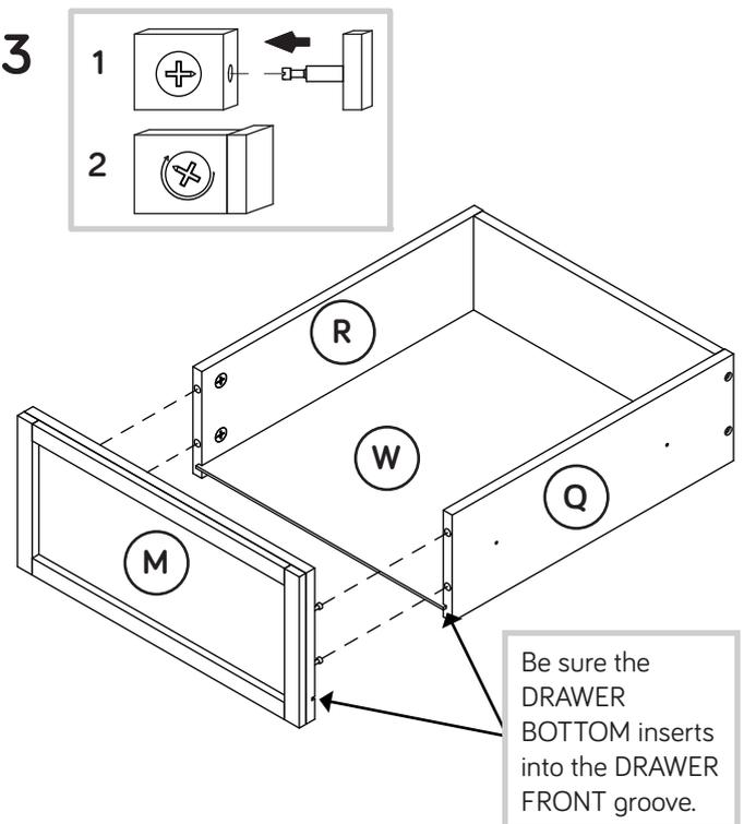
Fasten the SMALL RIGHT DRAWER FRONT (M) to the SMALL DRAWER SIDES (Q and R). Tighten four HIDDEN CAMS.
