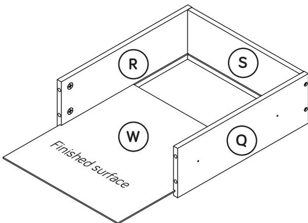
Slide the DRAWER BOTTOM (W) into the grooves in the SMALL DRAWER SIDES (Q and R) and SMALL DRAWER BACK (S).
