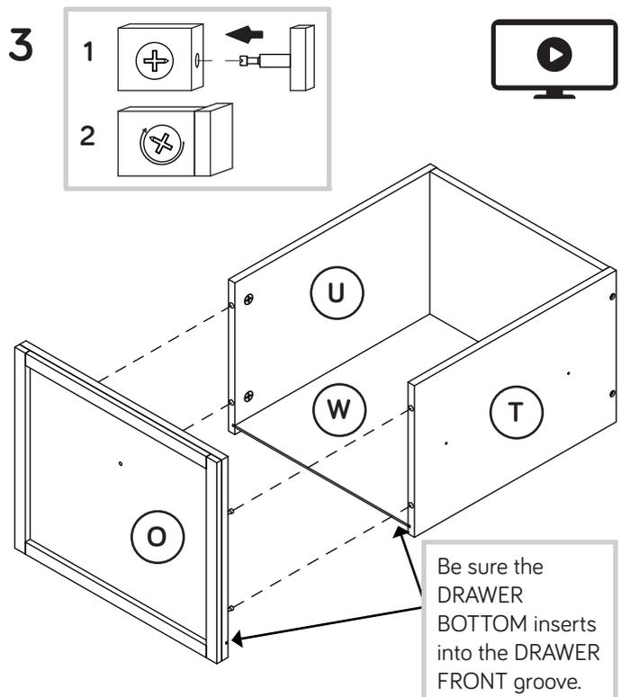
Fasten the LARGE RIGHT DRAWER FRONT (O) to the LARGE DRAWER SIDES (T and U). Tighten four HIDDEN CAMS.
