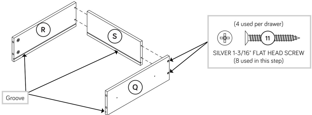
Fasten the SMALL DRAWER SIDES (Q and R) to the SMALL DRAWER BACK (S). Use four SILVER 1-3/16" FLAT HEAD SCREWS (11).
