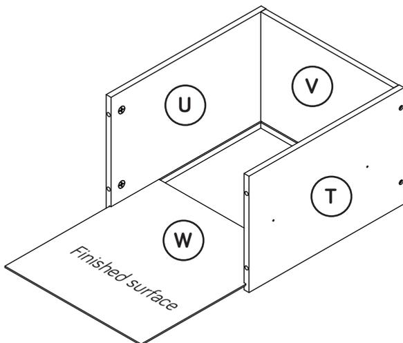
Slide the DRAWER BOTTOM (W) into the grooves in the LARGE DRAWER SIDES (T and U) and LARGE DRAWER BACK (V).
