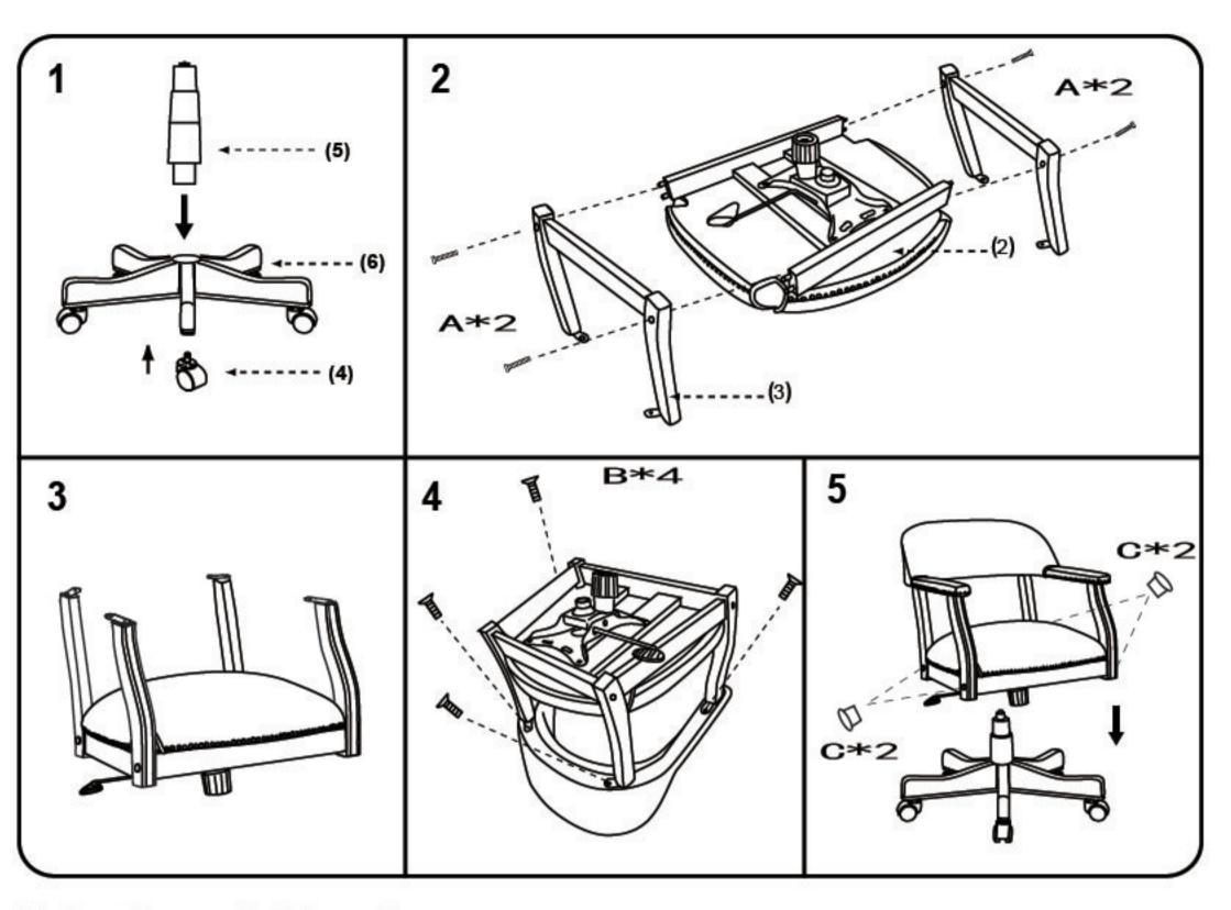
Note: Please tighten all arm screws using allen key before step 5
