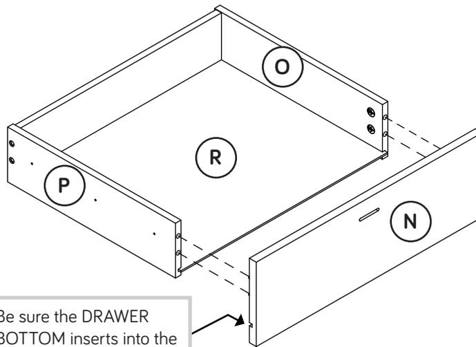
Be sure the DRAWER BOTTOM inserts into the DRAWER FRONT groove.
