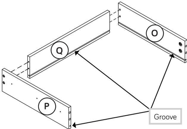
Fasten the DRAWER SIDES (O and P) to the DRAWER BACK (Q). Use four BLACK 1-1/2" FLAT HEAD SCREWS (16).
