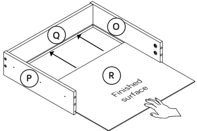
Slide the DRAWER BOTTOM (R) into the grooves in the DRAWER SIDES (O and P) and DRAWER BACK (Q).
